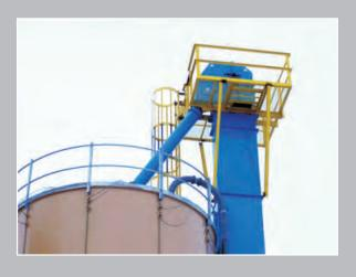
drum. Bucket elevators with chain transmission are generally equipped with two parallel transmission chains, and there are a pair of transmission chain top or down and a pair of redirection sprocket down or top. Bucket elevator are generally equipped with chassis to prevent the dust will be blew in bucket elevator.
